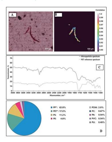
Figure 1: FT-IR microspectroscopy and spectral correlation analysis were used to characterize microplastics.
